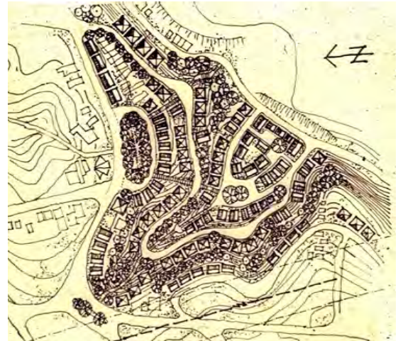
Alternative design for the upgrading of the informal settlement Van Van on hilly terrain outside Santiago de Cuba. Similar as in La Terrazas, individual family houses can be placed along the contour lines. Design: Kosta Mathéy
