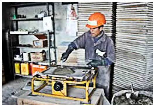
Tevi Cement tile production developed in the Technical University ISPJAE (Photo: Ecosur)
