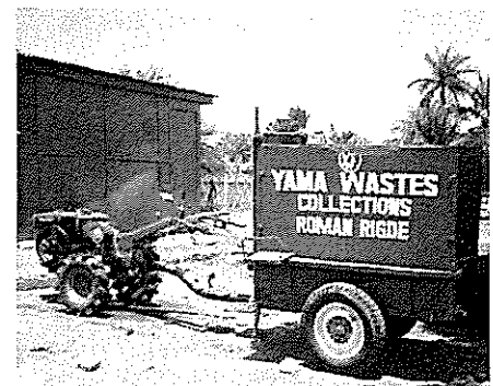
4. Powered tiller 40-50 houses/ trip, max. distance 5000 m
