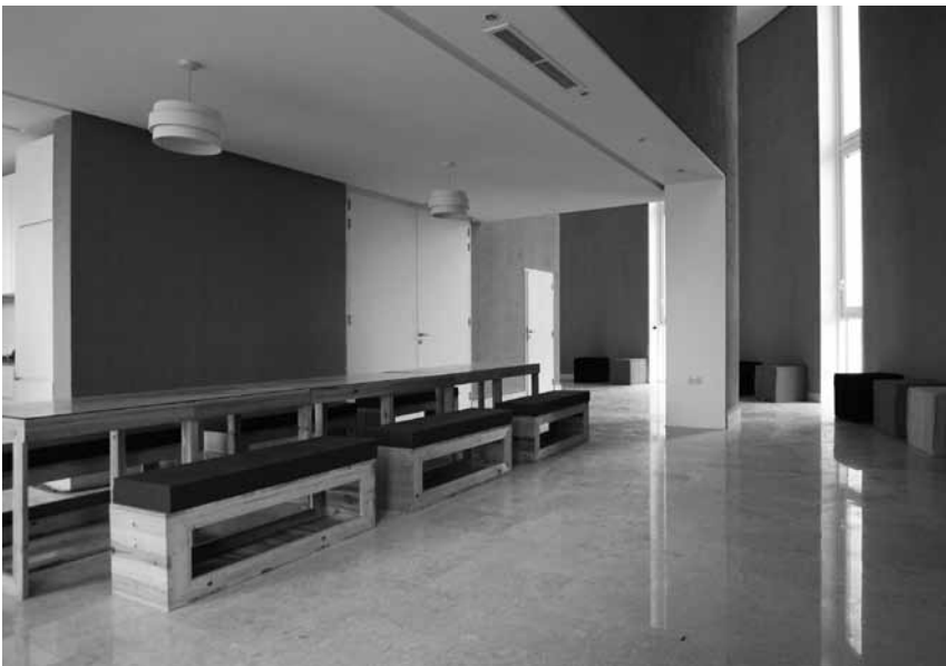
▼ Figure 5: For the ECOHAUS we selected local materials that perform best in the situation where we needed them. For example: mud bricks are a fantastic material for interior walls because – besides being fully recyclable – they have a high thermal mass, can buffer humidity, offer great acoustic qualities, and generally contribute to healthy air quality.
