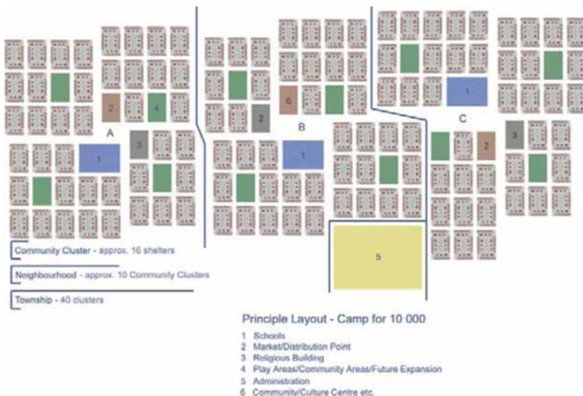
Figure 2: Groups of shelter clusters make up blocks. Source: Norwegian Refugee Council (2004) Camp Management Toolkit
