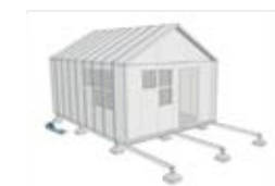
Step 7: Wrap and tighten liina around top and bottom of the walls
