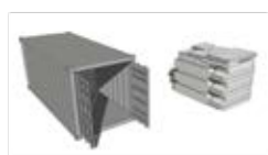
2 flat-pack shelters fit in a standard shipping container
