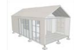
Step 9: Unroll canvas over shelter and attach to foundation beams
