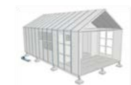
Step 8: Make and fit up terrace, attach 2 liina on roof ridge and terrace base
