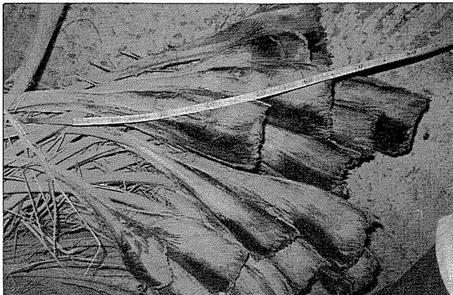
Fig. 2: Palm leaves including the broad, triangular part, i.e. the palm sheaths, which were used to infill ceilings and roofs.
